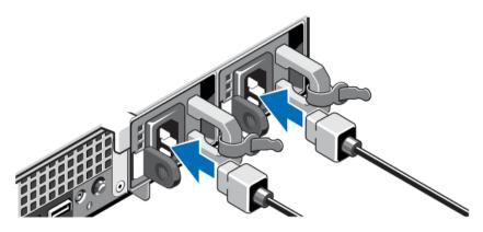
Figure 3. Connecting the Power Cable(s)
