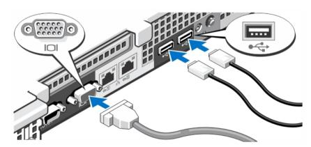
Figure 2. Optional—Connecting the Keyboard, Mouse, and Monitor
