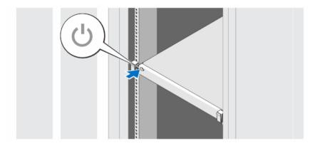
Figure 5. Turning on the System
