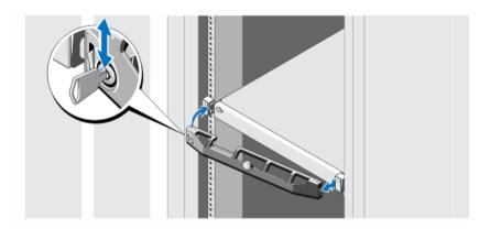
Figure 6. Installing the Optional Bezel
